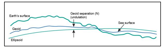
Consequently, two main reference surfaces have been established to approximate the shape of the Earth.
