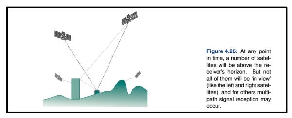
4. Errors related to relative geometry of satellites and receiver - GDOP error
