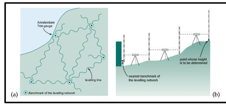
Figure 4.3: A levelling network implements a local vertical datum: (a) network of levelling lines starting from the Amsterdam tide-gauge, showing some of the benchmarks; (b) how the orthometric height (H)is determined for some point, working from the nearest benchmark.
