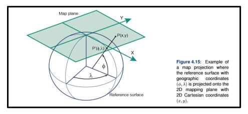
The actual mapping cannot usually be visualized as a true geometric projection, directly onto the mapping plane. This is achieved through mapping equations.
